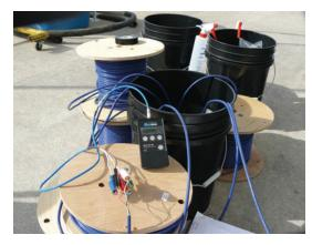
Figure 6-5 Presoaking the Vibrating Wire Transducers
