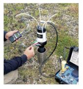
Figure 7-1 Testing Pumps and Transducers
