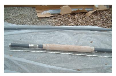
Figure 4-3 A Base Plug, Casing, Port, and Packer Section
