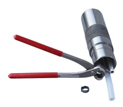
Figure 6-3 Tubing attached to Port Stem Using Oetiker Clamp
