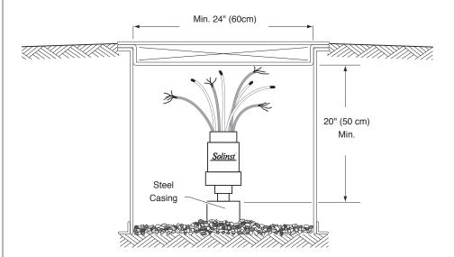
Figure 9-4 Waterloo Multilevel Wellhead Inside Flushmount Vault
