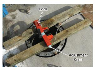
Figure 4-2 An Installation Clamp Over a Borehole
