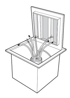
Figure 9-5 Typical Road Box or Vault
