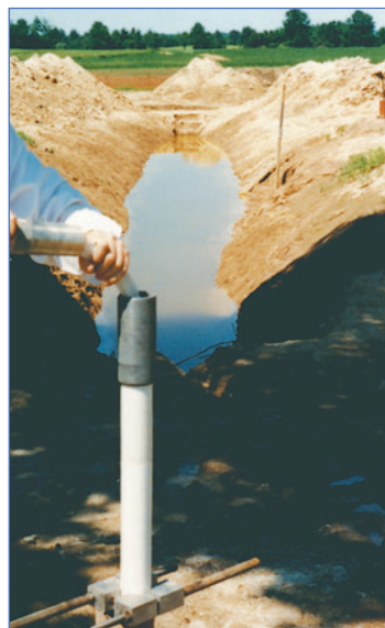
Underground oil pipeline leak assessment. Three 150 ft. (45m) installations. Two point rising head permeability tests were conducted in each interval of the Multilevel System. (See diagram showing contaminant distribution at left.)
