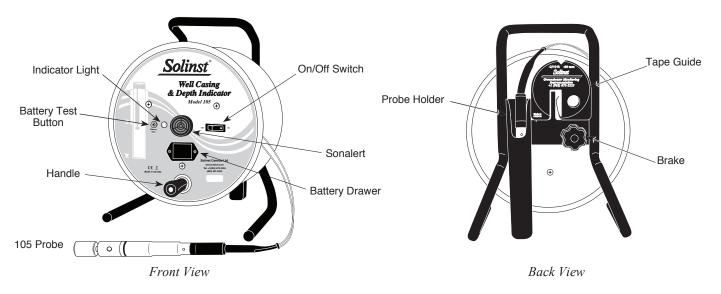
Well Casing Detection: Quick intermittent beeps and flashing red light.
